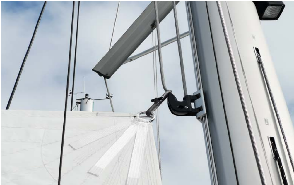
Pic 4. Loop not engaging hook.
