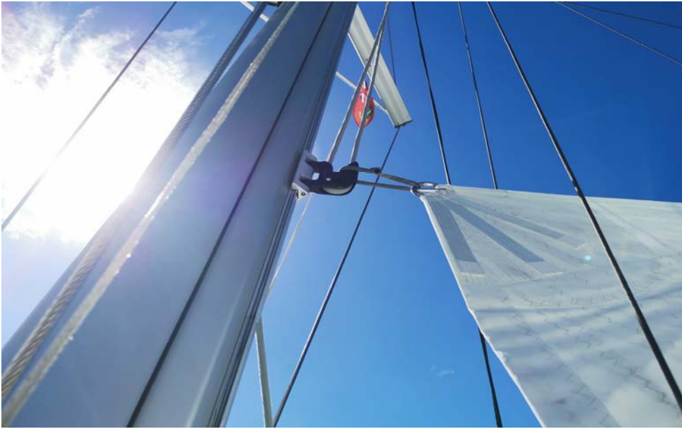
Pic 3. Looped line sitting on Halyard hook
